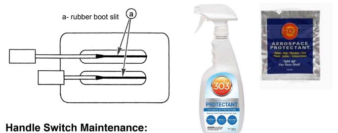
IMPORTANT: If salt build up or sticking is observed on the handle switches, rinse the affected area with fresh water and apply a water displacing lubricant.
