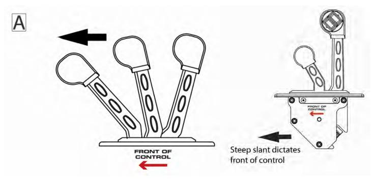
A) Forward cant models; arrow pointing to the ship's bow
