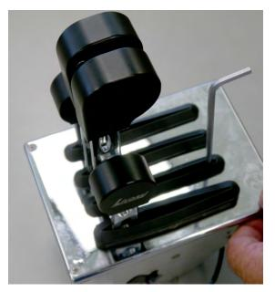
4. Turn clockwise to increase friction / detent. Turn counter clockwise to decrease friction / detent
